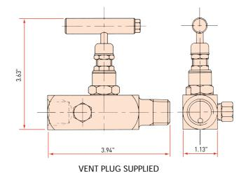
Gauge multiport valve Male inlet x three Female outlets
