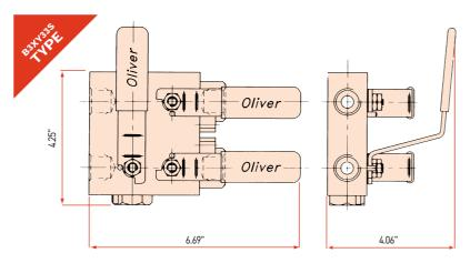
Three valve remote mount pipe to pipe manifold for isolation of process and equalising of instrument.
