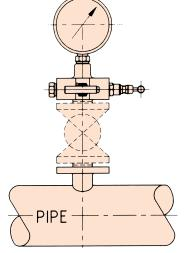
easy installation after an existing primary isolate valve. Dual instrument connections enable instrument to be mounted vertically on either horizontal or vertical line mounting application
