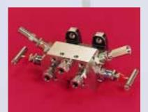
Used for differential pressure, this is the most commonly used four valve manifold and constitutes one isolate valve for the high side, one isolate valve for the low side, one equalise valve and one single vent valve. The isolation valves are Tee bar operable, the vent and equalise valve each have anti tamper head units. By equalising the valve you are able to vent both sides.
