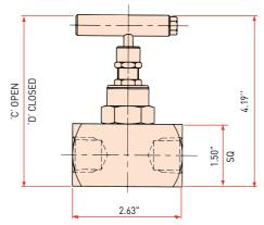
Note:  $^{1}/_{4}$ ",  $^{3}/_{8}$ " and  $^{1}/_{2}$ " NPT threads rate to 10,000 PSI only  $^{3}/_{4}$ " and 1" NPT threads rate to 6,000 PSI only
