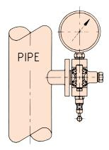
VERTICAL PIPING PRESSURE MEASUREMENT
