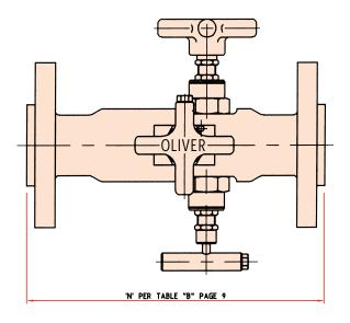
FLANGE TO PIPE – ONE BORE – THREE STANDARD MATERIALS
