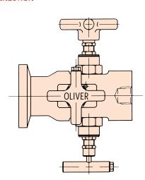
Any make or size of "Pipe Clamp Lock Connection" can be accommodated on the standard D, F or N type Double Block and Bleed Valves (N type shown) and also on the larger Twinsafe Valves.
