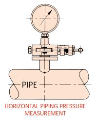
Slimline can be installed as the primary isolate valve, in either single block, block and bleed or double block and bleed versions. Dual instrument connections enable instrument to be mounted vertically on either horizontal or vertical line mounting application.
