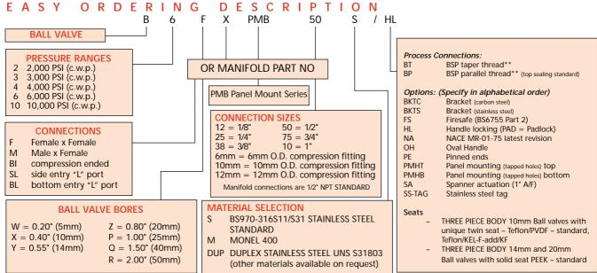
IMPORTANT NOTE – Always refer to table on page 21 to make sure that the required connection size, pressure rating and bore size are available. 23
