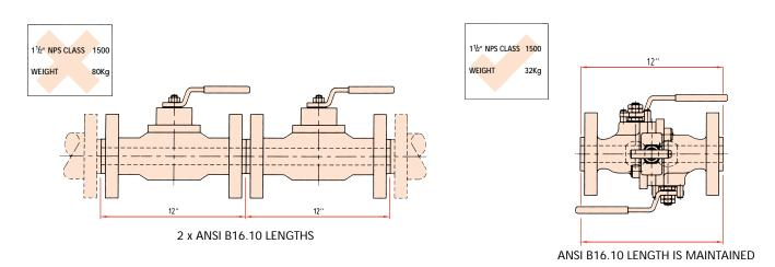
Twinsafe® DBB can be retrofitted in the space of a single ANSI standards length valve.
