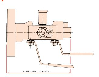
FLANGE TO PIPE - TWO BORES - THREE STANDARD MATERIALS
