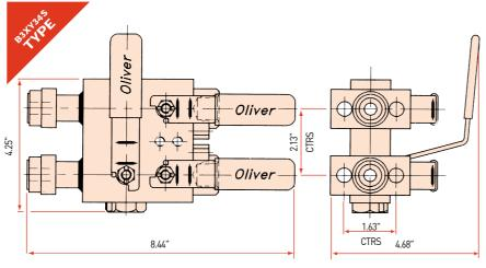
Three valve direct mount pipe to flange manifold for isolation of process and equalising of instrument.
