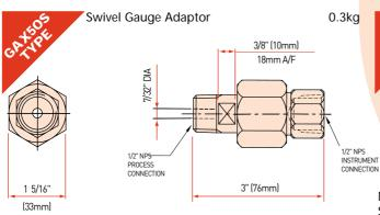
Metal Seals 540°C Max Temperature 10,000 PSI Max Pressure Standard Material 316 stainless steel **Standard Connections** 1/2" NPT Male x Female
