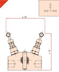
needle pattern valves arranged for double block and bleed of instrument.
