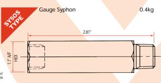
Max Pressure 6,000 PSI Standard Material 316 stainless steel **Standard Connections** 1/2" NPT Male x Female
