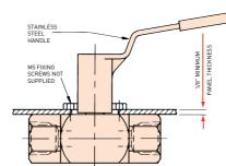
For all three piece body sizes this simple, and cost effective bossless solution is a clear advantage. Handle locking and oval handle not available.
