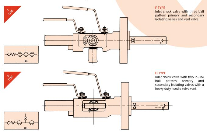
FLANGE SIZE 11/2" NB, FLANGE CLASSES 150 TO 2500 RF & RTJ. OPTION, FLANGE SIZE 2" NB, FLANGE CLASSES 150 TO 2500 RF & RTJ. OTHER BALL VALVE BORE SIZES AND FLANGE SIZES CAN BE ACCOMMODATED.
