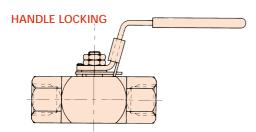
Valves can be locked in either the open or closed position with padlock available
