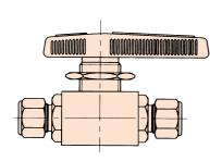
Panel mount "PMB series" three piece 6,000 PSI range ball valves. Coloured handles – black standard, options – red (RD), green (GR), blue (BL), yellow (YL), orange (OR) or stainless steel (HSS). Range of end connectors as standard and NACE option.
