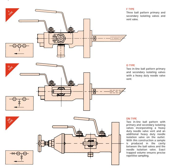
FLANGE SIZE 11/2" NB, FLANGE CLASSES 150 TO 2500 RF & RTJ. OPTION, FLANGE SIZE 2" NB, FLANGE CLASSES 150 to 2500 RF & RTJ. OTHER BALL VALVE BORE SIZES AND FLANGE SIZES CAN BE ACCOMMODATED.
