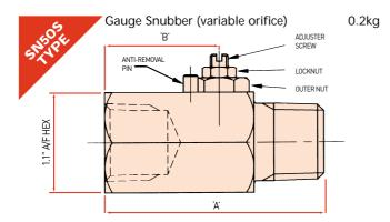
Seals VITON Max Temperature 120°C Max Pressure 6,000 PSI
