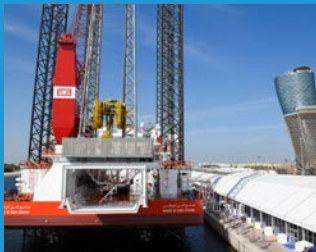
GMS – GULF MARINE SERVICES EVOLUTION CANTILEVER SELF- PROPELLED SELF-ELEVATING WELL INTERVENTION BARGE
