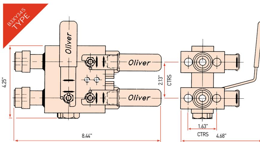
Three valve direct mount pipe to flange manifold for isolation of process and equalising of instrument. Available in 3,000 PSI pressure range with 10mm bore. Standard inlet connections 1/2" NPT (female).
