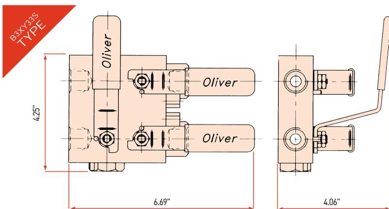
Three valve remote mount pipe to pipe manifold for isolation of process and equalising of instrument. Available in 3,000 PSI pressure range with 10mm bore. Standard connections 1/2" NPT (female).
