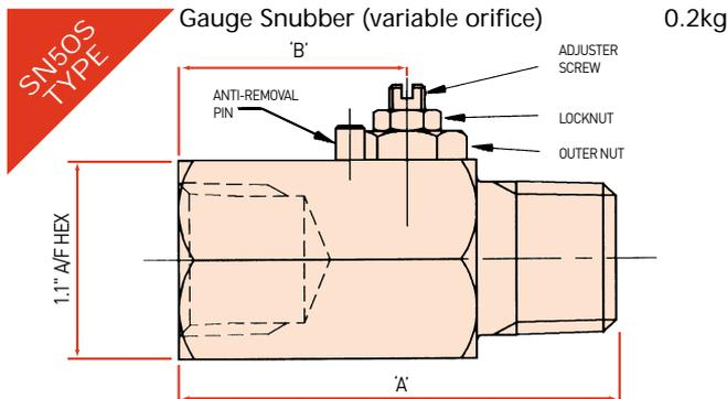
**Gauge Snubber (variable orifice)** 0.2kg
