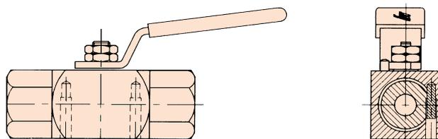
This simple but effective patented solution totally eliminates any possibility of inadvertent removal of end connector pieces by operator or vibration whilst in service.
