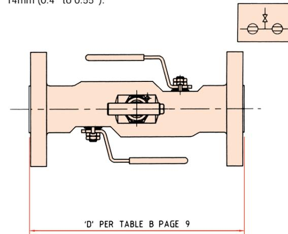
FLANGE TO PIPE – THREE BORES – THREE STANDARD MATERIALS
