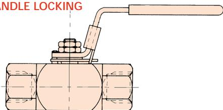
Valves can be locked in either the open or closed position with padlock available
