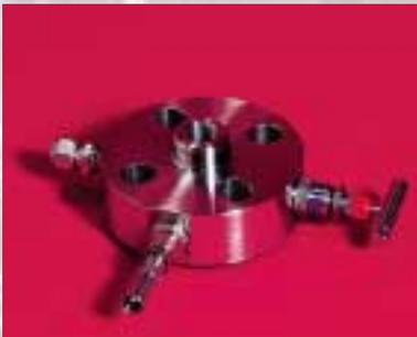
Although pressure gauges could be used on the isolate/vent block as depicted earlier, commonly, pressure gauges are screwed to a Monoflange. There are two types of monoflanges, both being block and bleed and having a Tee bar operable isolation valve and an anti tamper vent valve.
