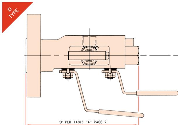
This all forged manifold comprises two in-line ball primary and secondary isolating valves with a heavy duty needle valve vent. Offering through to process rodding in bore sizes from 10mm to 14mm (0.4" to 0.55").
