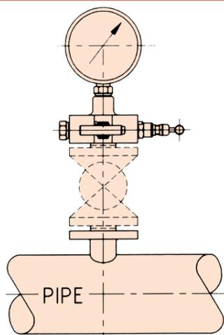
HORIZONTAL PIPING PRESSURE MEASUREMENT
