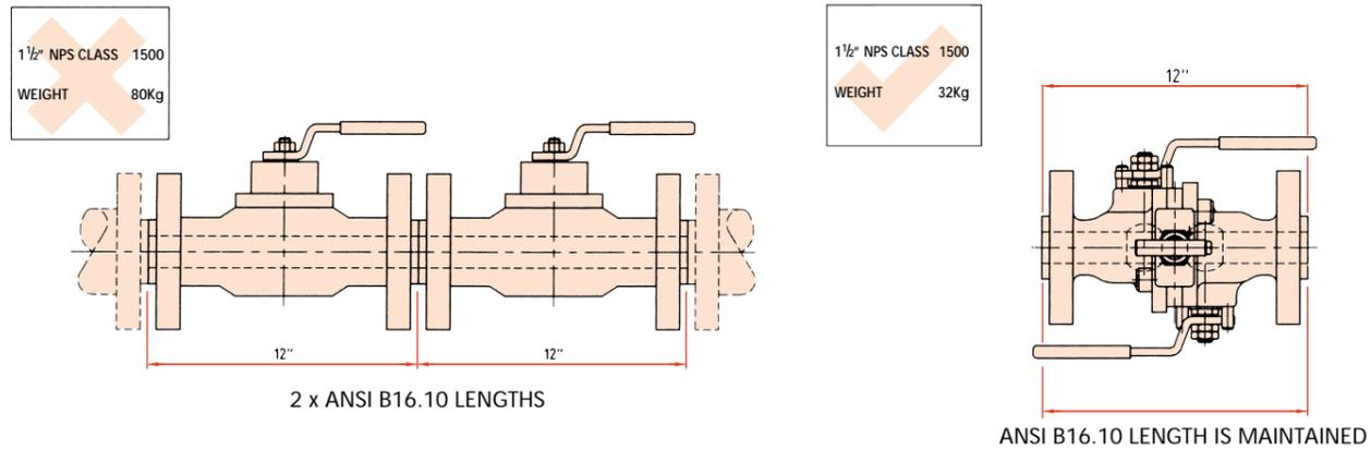
Twinsafe® DBB can be retrofitted in the space of a single ANSI standards length valve. Oliver double block and bleed isolating valves offer the same solution at dramatically REDUCED COST with the equivalent benefit of LOW WEIGHT and SPACE SAVING, added to the EASE OF INSTALLATION and potential for direct replacement in existing installations without the need for pipework modifications or lengthy and expensive plant shutdowns
