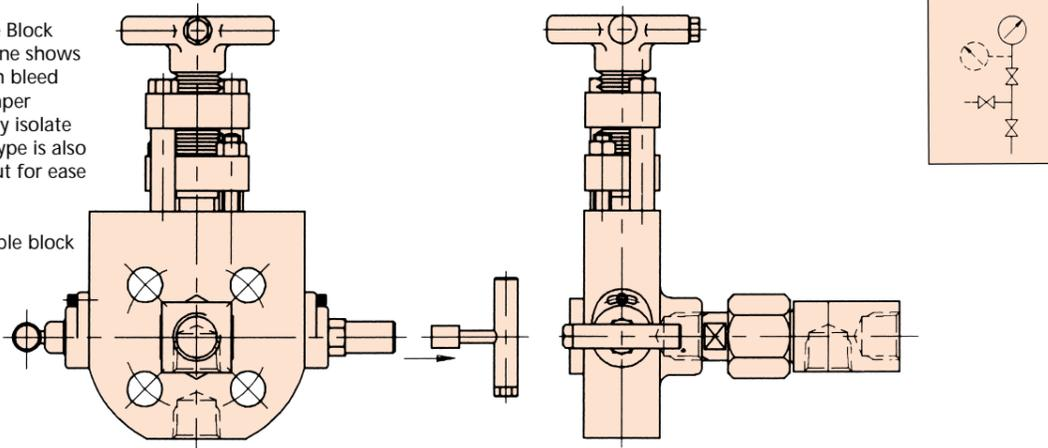
This standard configuration of Double Block and Bleed Style Slimline is shown with standard needle valves for bleed and secondary isolation.
