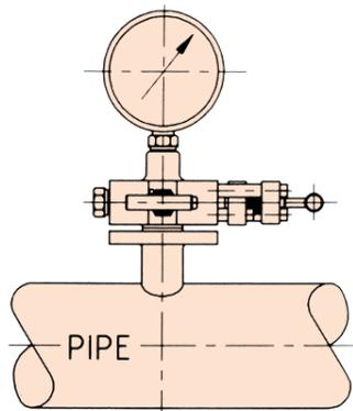
HORIZONTAL PIPING PRESSURE MEASUREMENT
