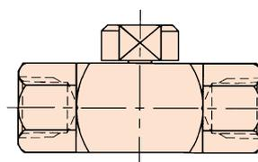
With Spanner actuation the valve is operated using a 1" A/F spanner, reducing tapering and accidental operation.
