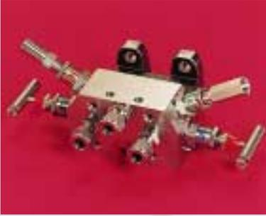
Used for differential pressure, this is the most commonly used four valve manifold and constitutes one isolate valve for the high side, one isolate valve for the low side, one equalise valve and one single vent valve. The isolation valves are Tee bar operable, the vent and equalise valve each have anti tamper head units. By equalising the valve you are able to vent both sides.
