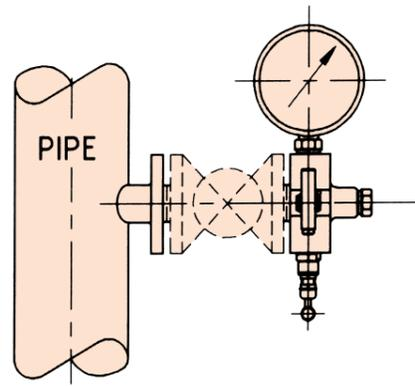
VERTICAL PIPING PRESSURE MEASUREMENT
