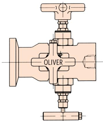
Any make or size of "Pipe Clamp Lock Connection" can be accommodated on the standard D, F or N type Double Block and Bleed Valves (N type shown) and also on the larger Twinsafe Valves.
