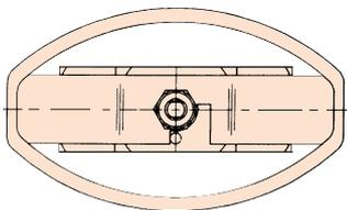
An oval handle can be fitted as an option to the standard lever style (Plan view shown).
