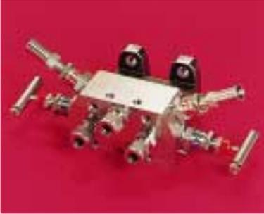
This four valve manifold is designed for particular applications where the contamination of both process streams are not permitted. There is no equalise valve, but in its place there is a further vent valve, to allow the isolation and venting of both sides independently. The isolation valves are Tee bar operable, the vent valves each having anti tamper head units.
