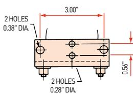
For mounting 2, 3 & 5 valve manifolds to a 2" NB pipestand. Mounting brackets to a 2" NB pipestand with "U" bolts, washers and nuts. Material of all components is zinc plated and passivated Carbon Steel. Special brackets can be supplied on request.
