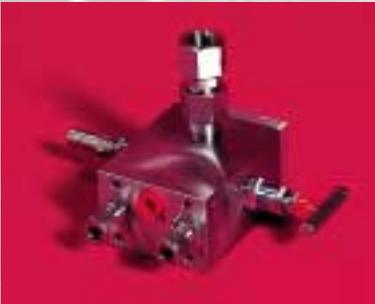
This is the manifold which has been provided for the Gauge, Switch and Gauge Pressure Transmitters which have a screw instrument connection. There are three versions available; 1/2" NPT female, 1/2" NPT male and G1/2" parallel female. The isolation valve is Tee bar operable, the vent valve having anti tamper head unit.
