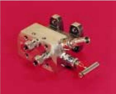
There are two versions of this manifold available, the most common is the manifold suitable for the Gauge Pressure Transmitter with traditional flanged mounting. The other manifold is provided for Differential Pressure Transmitters which are used typically in level applications where the low pressure side is vented to atmosphere. The isolation valve is Tee bar operable, the vent valve having an anti tamper head unit.
