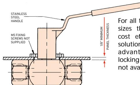
For all three piece body sizes this simple, and cost effective bossless solution is a clear advantage. Handle locking and oval handle not available.
