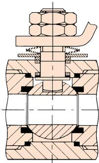
Tested to BS6755 part 2, these valves have body and stem seals in fire resistant Grafoil. The metal lip seat is designed to ensure leak free seating when the PTFE burns in fire conditions. The spindle disc springs ensure a positive leak-free gland.
