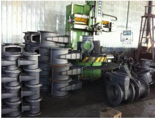
Vertical lathe mainly use for machining oversize valve bodies.
