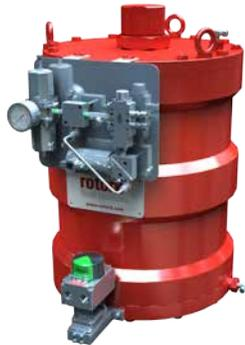
The CQ self-contained actuator is a fully concentric design based on a helical mechanism, transforming the linear motion of the piston into a quarter-turn rotation of the valve stem.
