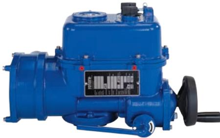
The Q range is a single-phase part-turn direct drive electric actuator available in two versions, both environmentally sealed to IP68. Q standard for simple open / close duties where on / off control is required and the Q Pak which incorporates a specially designed control interface module enabling operation from a variety of remote control signals.
