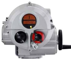
The IQTF provides extended output rotation for part-turn valve types requiring more than 90° for operation. Typical valves include 180° and 270° diverter valves and multiport manifolds requiring bi-directional 360° operation. The IQTF actuator has a low output speed for increased positional accuracy and may also be utilised for low turn, multi-turn applications where slow operation is required. Additional features listed on p7.
