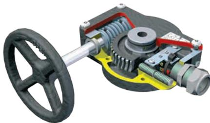
Quarter-turn cast iron gearbox suitable for use with fire protection (i.e. sprinkler) systems, includes limit switches to be incorporated into a supervisory electrical circuit. Designed and tested specifically to meet UL1901 specification and FM1112 Approval.
