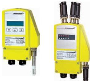
ExCos modulating sensors and ExBin binary switches are designed for use in hazardous areas. No additional modules in the panel required. No intrinsically safe wiring required. All parameters adjustable on site without additional tools or measuring devices. Sensors and switches for pressure, delta pressure, temperature and humidity available. Explosionproof design for all gases, mists, vapours and dust.
