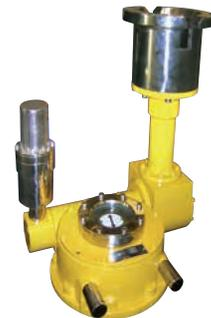
The WGS range of quarter-turn operators are designed for heavy-duty subsea applications at any depth with carefully chosen materials to offer the highest level of reliability required in this very harsh environment. The operators are equipped with membrane or piston type pressure compensators to balance the pressure and allow them to work at any depth.
