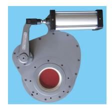
The pneumatic ceramic rotary gate valve is developed according to the fault frequently occurred during the operation of the dome valve .The ceramics is used as the wear-resisting parts.The sealing surface of the product is made of toughened engineering ceramics with good abrasion resistance and prolonged service life.They are widely use in dense phase pneumatic conveying system of power plant.
