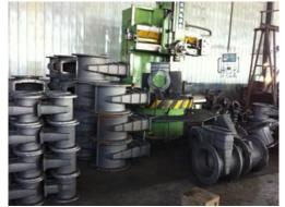
Vertical lathe lathe mainly use for machining oversize valve bodies.
